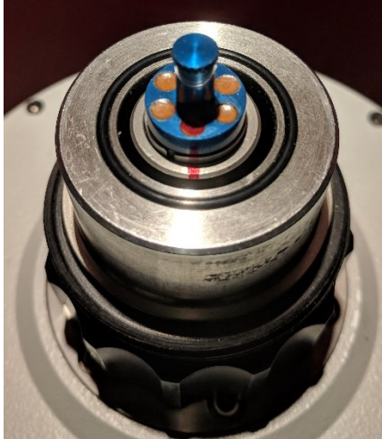
Figure 2. Alignment marks to ensure the same rotational position of the sample rod to minimize any radial offsets of the sample and sample holder within the gradiometer.
